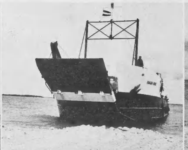
THE INAGUA Wave approaches Barcadera, left, and drops her unloading ramp, center, as she hits the beach. The low-boy rig, right and below, leaves the craft mostly under its own power.
